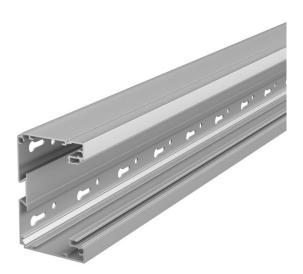
Device installation trunking with base perforation for direct wall mounting or mounting on panels. Other RAL colours can be supplied on request. The visible surfaces of the painted device installation trunking are laminated. The cover must be ordered separately.
