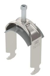
Clamp clip with hammerhead foot, plastic pressure sleeve made of polypropylene. For vertical and horizontal mounting of 1 single cable on a C-profile rail. For a slot width 16–17 mm. With 1-start screw thread on pressure sleeve, universal hexagonal screw head WAF10, with slot and cross recess. Suitable for assembly indoors and outdoors. We recommend the use of a counter-sleeve.
