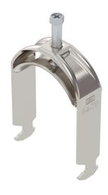
Clamp clip with hammerhead foot, metal pressure sleeve with rounded edges to protect the cable. For vertical and horizontal mounting of 1 single cable on a C-profile rail. For a slot width 16–17 mm. With 1-start screw thread on pressure sleeve, universal hexagonal screw head WAF10, with slot and cross recess. Suitable for assembly indoors and outdoors. We recommend the use of a countersleeve.
