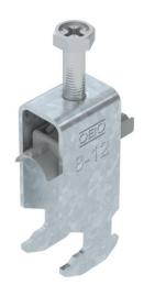
Clamp clip with hammerhead foot, plastic pressure sleeve made of polypropylene. For vertical and horizontal mounting of 2 single cables on a C-profile rail. For a slot width 16–17 mm. With 1-start screw thread on pressure sleeve, universal hexagonal screw head WAF10, with slot and cross recess. Suitable for assembly indoors and outdoors. Multiple cables should be separated by double sleeves. We recommend the use of a counter-sleeve.
