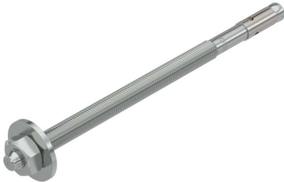
Bolt tie BZ3 for the anchoring of medium-duty to heavy-duty loads, both in cracked and non-cracked concrete. Suitable for heavy loads with small edge and axial distances. For knocking in.
