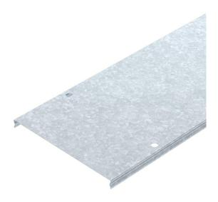
Lockable cover for mesh cable trays of type GR and GRM. Protects cables from damage, contamination and moisture from above. Suitable for industrial areas such as mechanical engineering. With transverse bead from 400 mm width.
