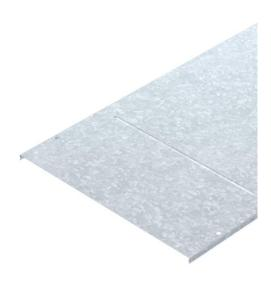
Lockable cover for mesh cable trays of type GR and GRM. Protects cables from damage, contamination and moisture from above. Suitable for industrial areas such as mechanical engineering. With transverse bead from 400 mm width.
