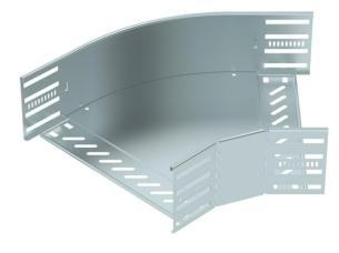
45° bend for the creation of a horizontal branch, fitting for lock and screw-on cable trays of side height 110 mm. Screwless mounting with double clamps or screw connection with FRS truss-head screws and M6 combination nuts. Can be used in indoor areas. Fastening material must be ordered separately.
