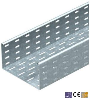
SKS 110 = Heavy-duty cable tray system with 110 mm side height. The cable tray is fastened to the bracket with bolts, type FRS M6 x 12. The surface coating is a coating created in a single-dip method with extra-high zinc thicknesses.
