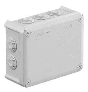
Junction box for the connection of cables and lines indoors and in protected outdoor areas. Rectangular design with plug-in seals to the sides and knock-out entries in the bottom. Suitable for wall and ceiling mounting and on mounting panels. With the option to fasten inside and to mount via the corner domes. Cover with quick lock, sealable. Made from halogen-free and UV-resistant materials.
