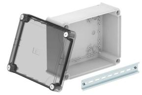
Closed junction box for the connection of cables in indoor and protected outdoor areas. Rectangular design without entries. Suitable for wall and ceiling mounting, on mounting panels and threads in the floor. With the option of fastening inside and to mount via the corner domes. High, transparent cover with quick lock, sealable. Made from halogen-free, UV-resistant materials.
