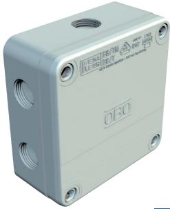
The B9/T... wet-room junction box comprises two different halogen-free plastic components, 2 additional entries in base with push-through membrane (for cable diameter up to 15 mm)
