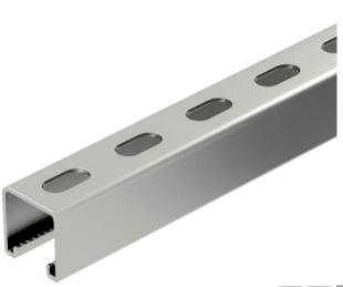
Heavy-duty C profile rail for individual installation of support constructions, e.g. for cable trays or as a panel for switchgear cabinets. Can also be used for cable routing, in conjunction with clamp clips with a U foot.
